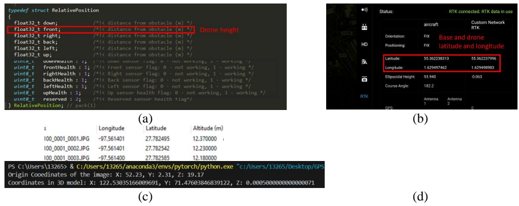
Figure 5: Localisation of defect via RTK subscription(a)(b), metadata of image(c) and coordinates conversion(d)
