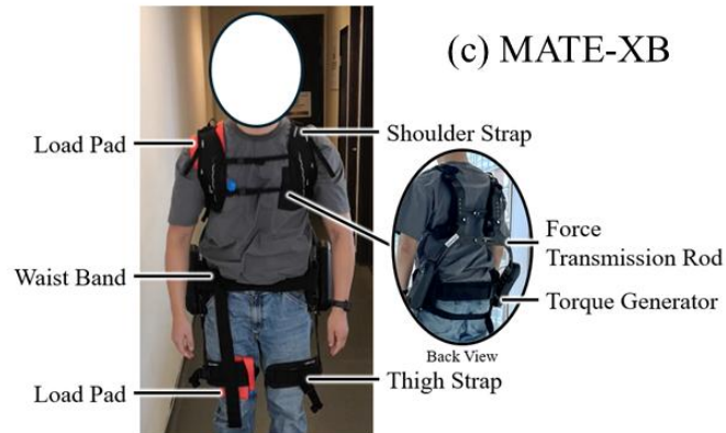
Figure 1: Main structures of the three compared exoskeletons and the installation positions of the load pads.
